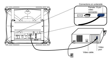
• Connect one end of the video cable to the video connector on your PC and the other end of the cable to the video connector on your monitor. Secure the cable by turning the thumbscrews on each connector.
